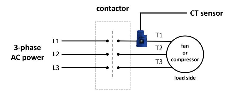
NOTE: Place clamp on load side. In case of multiple compressors then clamp on all compressor T1 lines. In case of multiple fans/blowers then clamp on all fan/blower T1 line.
